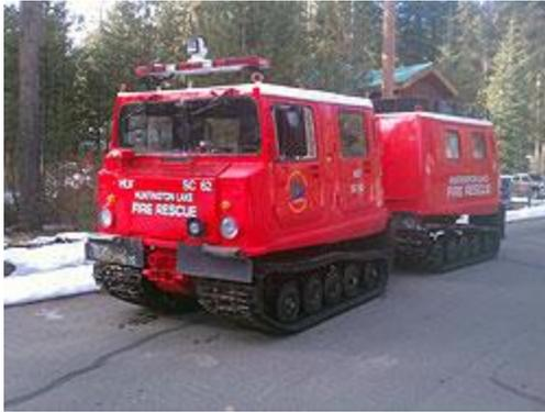
The Haggglunds snow-cat carries 13 and operates on pavement, dirt and gravel, ice and snow and can "swim" in rivers and lakes. With four driving tracks, the Haggglunds is capable of operating in the most severe winter conditions and has saved lives in the middle of winter.
